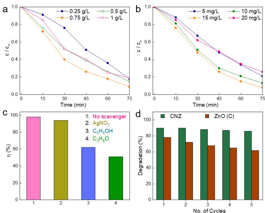
**Figure 6. (a) Effect of photocatalyst concentration over MB degradation, (b) Effect of MB concentration over degradation, (c) Effect of scavengers on the degradation of MB, and (d) Reusability measurements.**
