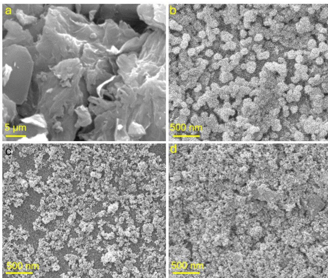
**Figure 3. SEM images of (a) g-C<sub>3</sub>N<sub>4</sub> nanosheets, (b) ZnO NPs, (c) NiO NPs, and (d) CNZ ternary nanocomposite.**
