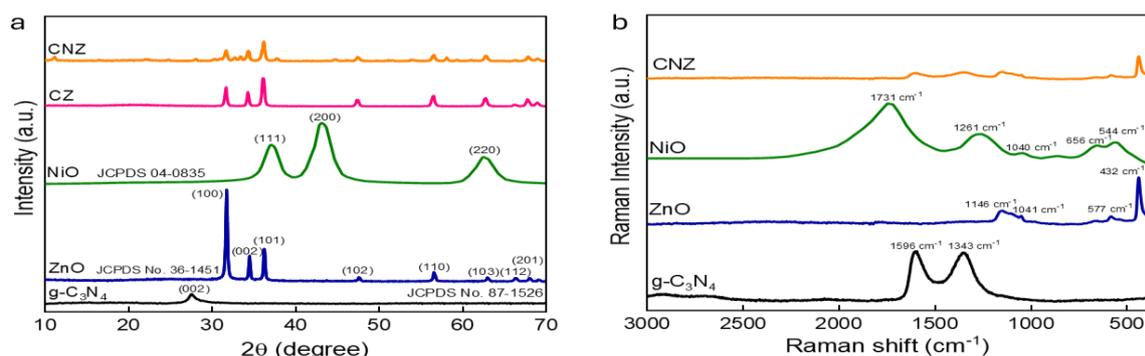
**Figure 2. (a) XRD patterns of g- $\text{C}_3\text{N}_4$ , ZnO, NiO, CZ, and CNZ photocatalyst, (b) Raman spectra of the g- $\text{C}_3\text{N}_4$ , ZnO, NiO, and CNZ photocatalyst**
