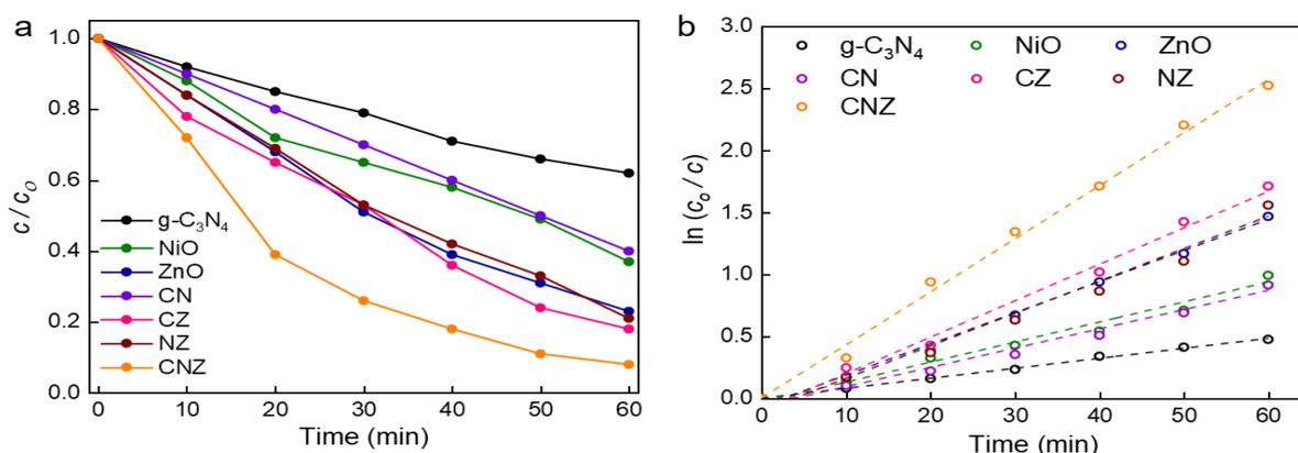
**Figure 5. (a) Photocatalytic activity of MB using g-C<sub>3</sub>N<sub>4</sub>, NiO, ZnO, CN, CZ, NZ, CNZ photocatalysts, (b) kinetic analysis of the same.**
