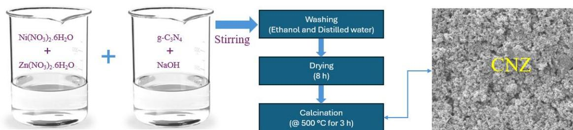
**Figure 1. Schematic illustration of the synthesis scheme for CNZ photocatalyst.**
