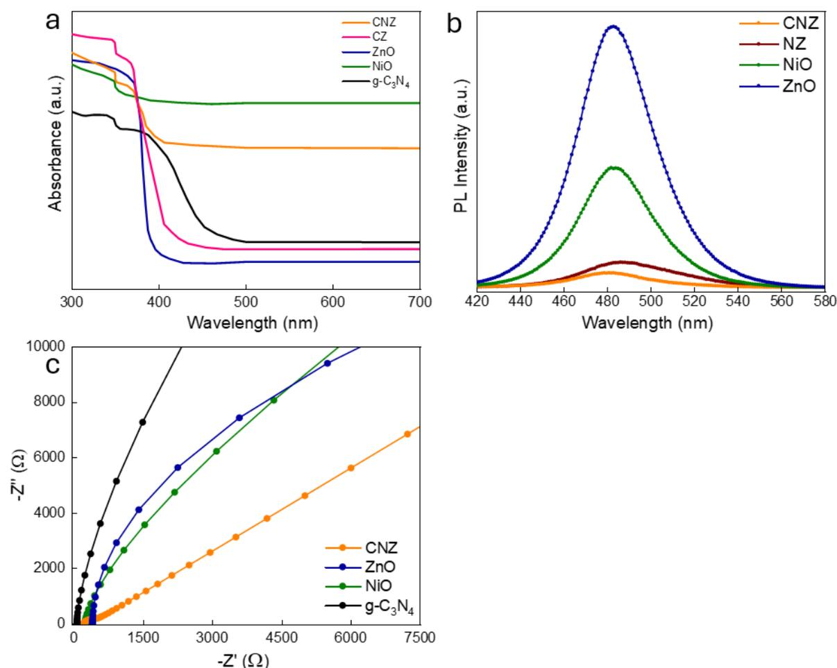
**Figure 4.** (a) UV-Vis absorbance spectra of  $g\text{-C}_3\text{N}_4$ , NiO, ZnO, CZ, and CNZ photocatalyst, (b) PL spectra of ZnO, NiO, NZ, and CNZ photocatalyst, and (c) EIS spectra of  $g\text{-C}_3\text{N}_4$ , NiO, ZnO, and CNZ photocatalyst.
