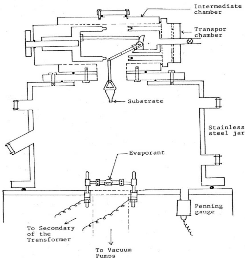
Fig. 1: Schematic diagram of vacuum evaporation assembly.
