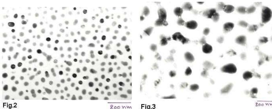
**Fig. 2:** Thin deposit of CsI after exposure to the atmosphere for 5 minutes.
