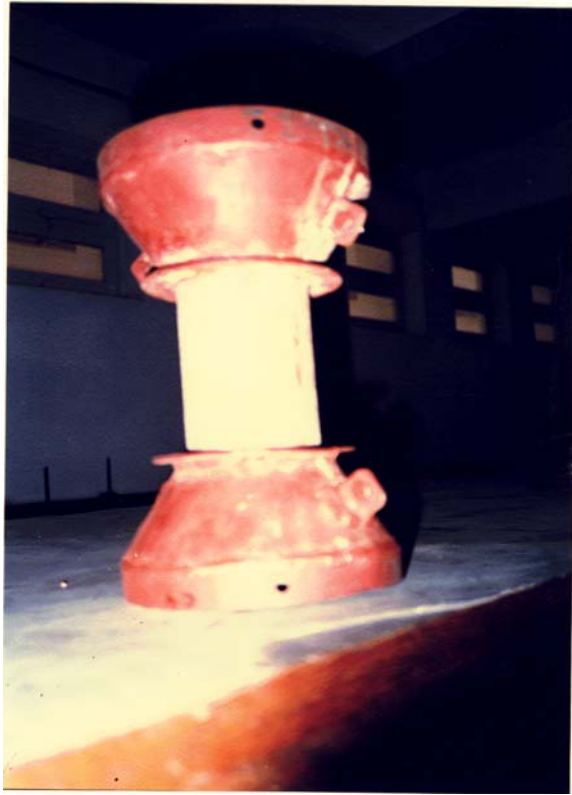
Fig. 5: Specimen ready for tensile testing.
