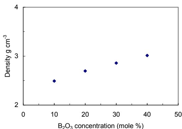
**Fig. 2:** Increase in mass density with the increasing concentration of B<sub>2</sub>O<sub>3</sub> in zinc-boro phosphate glasses.
