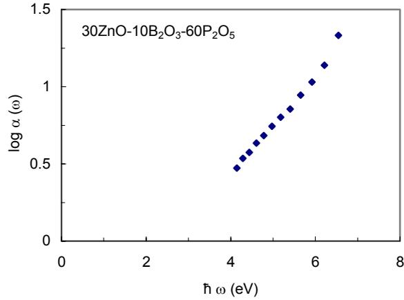
**Fig. 7:** A representative graph of  $\log \alpha$  vs  $(\hbar\omega)$  for the glass composition 30ZnO-10B<sub>2</sub>O<sub>3</sub>-60P<sub>2</sub>O<sub>5</sub>.
