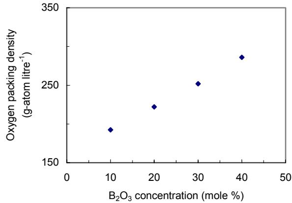
**Fig. 3:** Increase in oxygen packing density with the increasing concentration of  $B_2O_3$  in zinc-borophosphate glasses.
