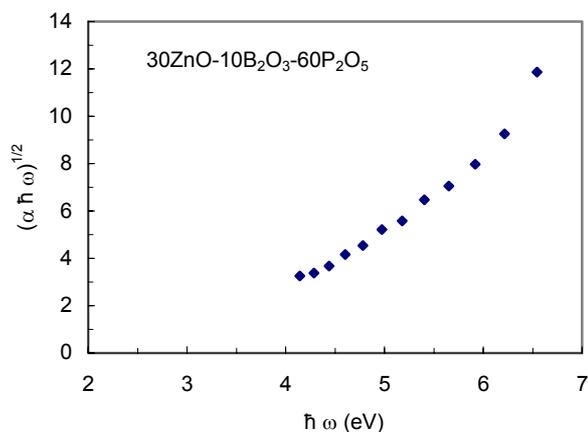
**Fig. 5:** A representative plot of  $(\alpha\hbar\omega)^{1/2}$  Vs photon energy ( $\hbar\omega$ ) for the glass composition 30ZnO-10B<sub>2</sub>O<sub>3</sub>-60P<sub>2</sub>O<sub>5</sub>.
