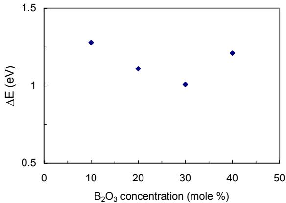
**Fig. 8:** Variation of  $\Delta E$  with the change in concentration of B<sub>2</sub>O<sub>3</sub>.
