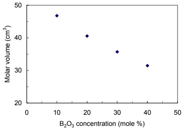
**Fig. 4:** Decrease in molar volume with the increasing concentration of  $B_2O_3$  in zinc-borophosphate glasses.
