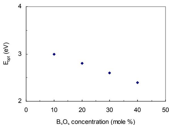
**Fig. 6:** Decrease in optical band gap with increasing concentration B<sub>2</sub>O<sub>3</sub> in zinc-borophosphate glasses.
