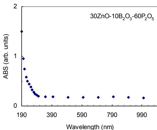
**Fig. 1:** A representative spectrum of absorption versus wave length (nm) for the glass composition 30ZnO-10B<sub>2</sub>O<sub>3</sub>-60P<sub>2</sub>O<sub>5</sub>.
